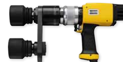
LTP 61 shut-off nutrunner with multi torque selector up to 4 different torque levels Torque range: 55 – 3,800 Nm Speed range: 50 – 1,800 rpm
